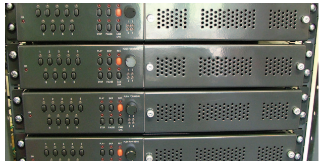
Slim Liberators are 1.5U high, but still have 4 hard discs removable from the front panel. Saves rack space, and they are low powered.
