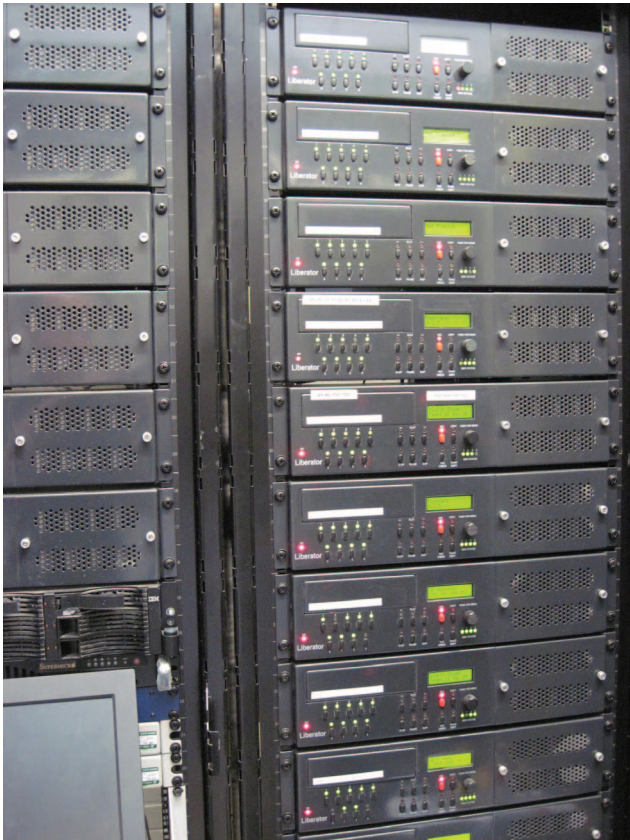
Part of a 230 camera system. Note because power consumption is so low, a 1U air space between recorders is not required. All hard disks are removable from the front panel.
